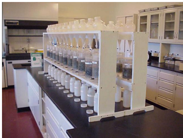
Fig. 1. Weekly rinsing of solutes from a suite of Duluth Complex rock samples tested using ASTM 5744-13e Option B at the Minnesota Department of Natural Resources Hibbing laboratory. 500 mL of deionized water is dripped from the separatory funnels onto the 1-kg rock samples and leachate is collected in the bottles below the humidity cells for subsequent analysis.
