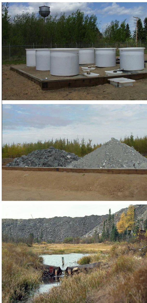
Fig. 6. The top two photos depict tank tests and test piles used for field dissolution testing of greenstone rock at the MN DNR Hibbing research site. The bottom photo depicts the weir at a site used for monitoring flow and water quality at the Dunka taconite mine in northeastern Minnesota.
